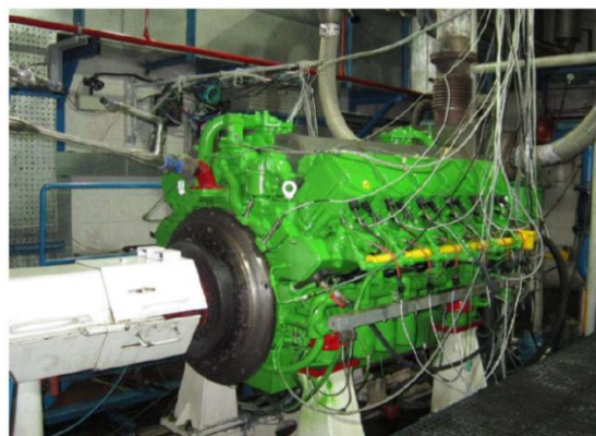
Figure 2: An overview of Iranian national heavy-duty diesel engine (D87) on the test bed (Jafari, Domiri Ganji, & Mirsalim, 2013).
