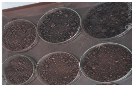
Figure 6. Comparison of bioremediation treatments after bacterial inoculation vs. control. Dark sample (top right) is contaminated soil without microbial inoculation (control).
