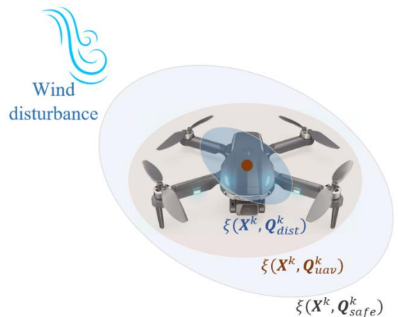
Fig. 2. The inner ellipsoid, \xi(\mathbf{X}^k, \mathbf{Q}_{dist}^k) , represents the ellipsoidal approximation of the FRSs. The middle ellipsoid, \xi(\mathbf{X}^k, \mathbf{Q}_{uav}^k) , and the outer ellipsoid, \xi(\mathbf{X}^k, \mathbf{Q}_{safe}^k) , represent the UAV ellipsoid and the safe ellipsoid, respectively.
